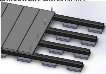
Attention: The WPC products' expansion rate is around 0.3% to 0.5% depends on deck length and weather condition in different places. Based on this expansion rate, there must be a gap (at least 3mm) always between two decks.
