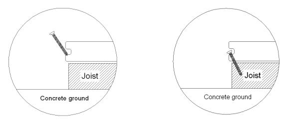
3C. Without starting clips, but screw from the top First, from the top of the deck, predrill a hole for the screw and into the joist; Second, fix the screw into the hole(see below pictures).
