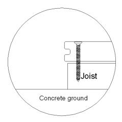
After the first deck is fixed, the rest decks to be fixed by screws and clips in turn
