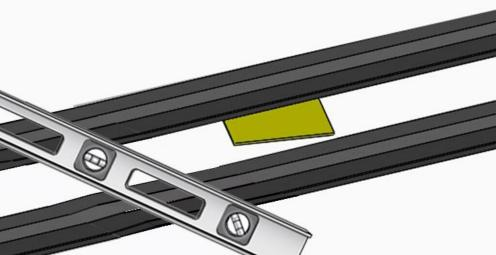
Attention: it is required that the deck surface is mounted flat and no water can collect on the surface or in the chambers. If water collects in the chambers for a long period, the board may start cupping and waving because of the moisture expansion.
